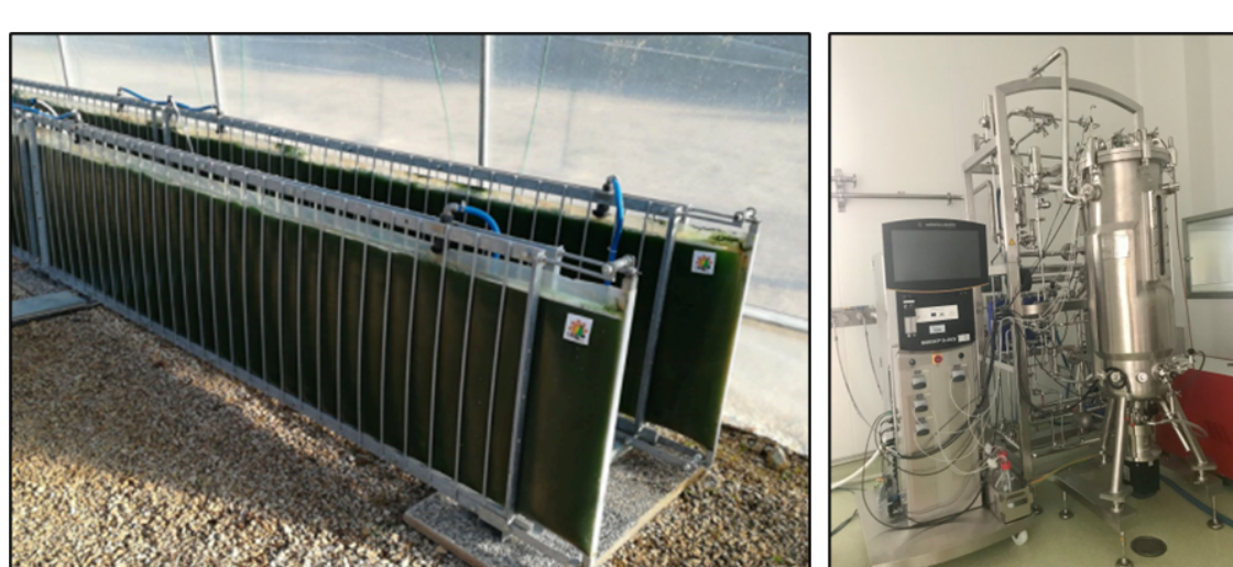
Figure 1. Image showing the types of reactor equipment that will be used to cultivate micro-algae under phototrophic (left) and heterotrophic (right) modalities at UCC.
